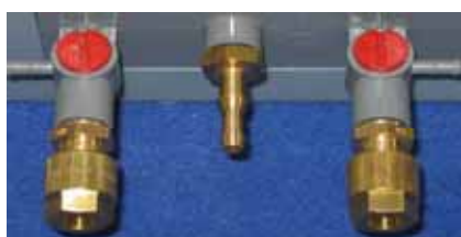
Connections for pipes
