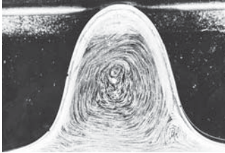
Spirally corrugated pipe: no dead-water zones, constant turbulence
